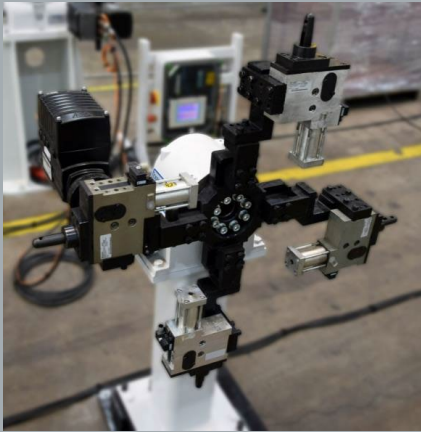
Application example: „Windmill“ - EGV-Trunnion as drive module for the flexible underbody clamping
