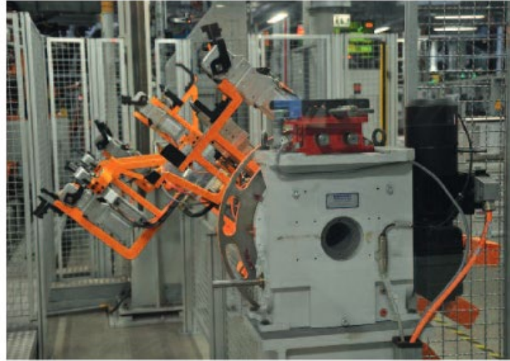
EXPERT Trunnion Drive Unit with maintenance looking device
