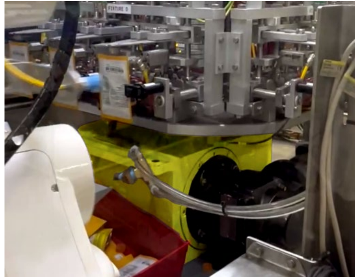
EXPERT Trunnion Drive Unit with maintenance looking device
