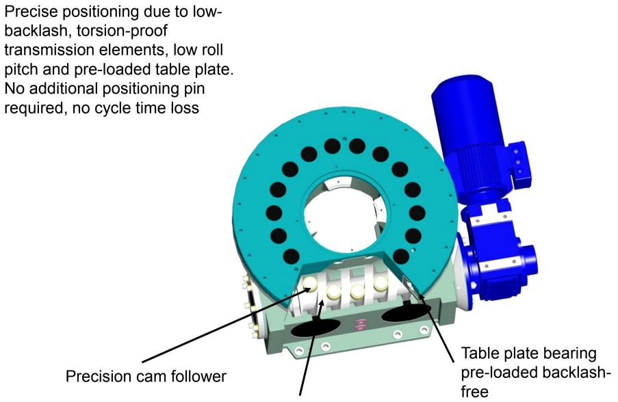
Restricted manufacturing tolerances of cam and table plate
